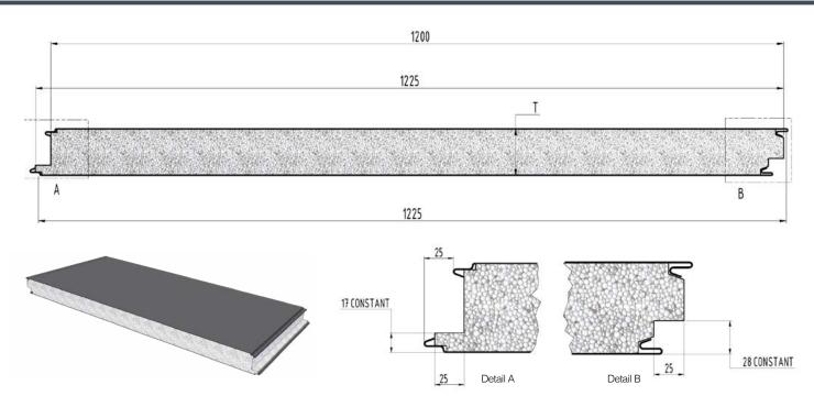
**DeltaSecretFix-EPS-FR** is an Insulated Wall Panel System, comprising of two pre-painted, roll-formed steel skins, bonded to a fire retardant grade expanded polystyrene core.
