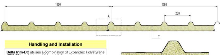
(EPS-FR) and Mineral Wool (MW) insulated core material. The fibrous structure of Mineral Wool makes it easy to fracture the woven fibres if handled and installed incorrectly. Please ensure that correct lifting equipment is used when the panels are transported and lifted into position. Refer to the Handling & Installation Manual - Roof Systems for the correct Crane & Sling Procedures.
