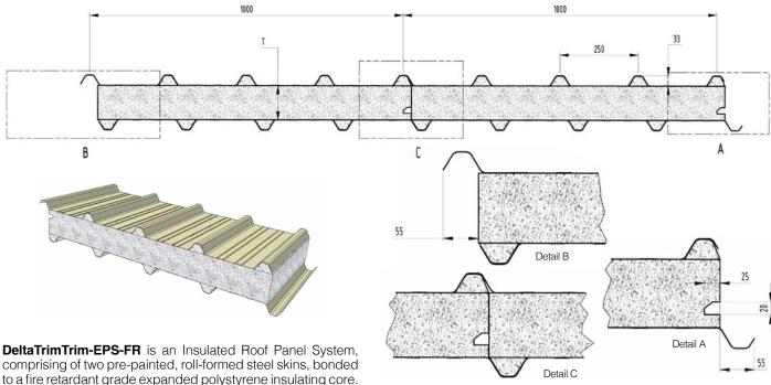
comprising of two pre-painted, roll-formed steel skins, bonded to a fire retardant grade expanded polystyrene insulating core.
