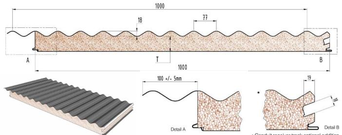
DeltaOrb-TPC is an Insulated Roof Panel System, comprising of two pre-painted, roll-formed steel skins, wbonded to a Thermosetting Phenolic Composite core.
